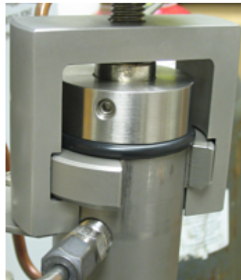
yoke turned counterclockwise and properly engaged
