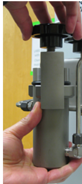
support the chamber to avoid pushing it down while turning the Hand Knob
