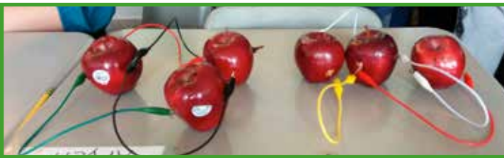
Fruit battery experiment: the apples were wired together and used to light up a small bulb.
