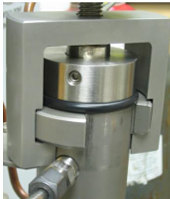
yoke turned counterclockwise and properly engaged
